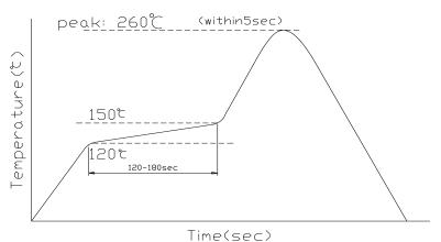
WAVE SOLDERING PROFILE FOR LEAD FREE PROCESS:
